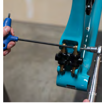
09. Use a ball-end wrench to prevent the inner Ti Female Bolts from rotating. Torque the 4x Flat Head Ti Male Bolts to 12.5 Nm .
