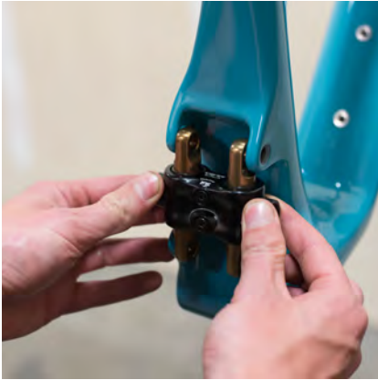
05. Push the SB100 Switch Infinity Link into the frame
