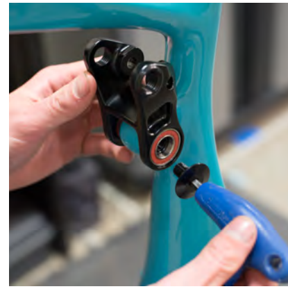
11. Install Male Link Pivot Bolt (300030293) into Female Link Pivot Bolt.
